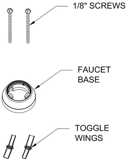
3. Assemble the 1/8" Screws & Toggle Wings into the Faucet Base. Adjust the Wings approximately 1" plus the thickness of the mounting surface away from the bottom of the Faucet Base.
