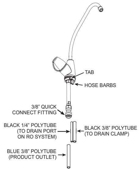
5. Connect the tubing to the Faucet. Push the Blue 3/8" Polytube into the 3/8" Quick Connect Fitting. Push the Black 3/8" Polytube onto the large Hose Barb. Push the Black 1/4" Polytube onto the small Hose Barb.
